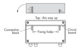
The circuit board can be slid out of the back box to make electrical connections easier.
