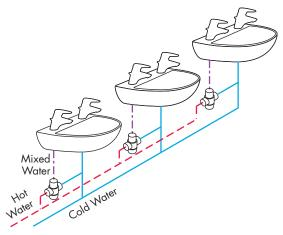
The Inta range of thermostatic mixing valves **MUST** be installed in an accessible position to ensure that maintenance, commissioning and testing of the **Inta Thermostatic Mixing Valves** can be undertaken easily.
