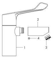
Periodically the spout and nozzle should be removed, cleaned and disinfected to remove any build up of debris, deposits or bio film which may affect the performance of the tap.
