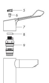
Isolate both the hot and cold water supplies Remove the indice (5), and unscrew retaining screw (6). Remove the handle (7) and the temperature stop ring (8). Using a suitable spanner unscrew the cartridge (9).
